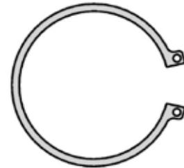
1-1/4" B Station Stripper Retaining Ring
