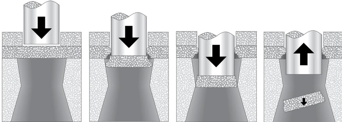
Material held securely by stripper before punch makes contact.
