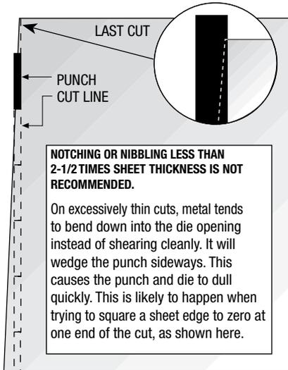
The Ultra clamp clearing slitting tool is designed to overcome these side load and twisting pressures. The advantage comes from punch point guiding. By squarely and tightly controlling the punch point where it contacts the sheet, the punch can accurately pierce a hole, even when punching partial hits.
