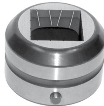
Mate Slug Free Light™ notches are cut at an angle to create a series of protrusions on the slug. As the slug moves through the die, the protrusions become trapped against the die land to prevent the slug pulling back on to the sheet. (Image enhanced for additional clarity)
