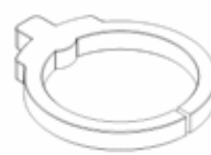
1-1/4" B Station HP (Series 90) Style Punch with hook ring Anti-Rotation Clip AOVBWBAC**
