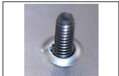
Photo 2: Shows the completed form, with a 10-24 machine screw.
