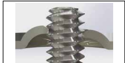
Figure 1: Cross sectional view of the sheet metal, produced using the hybrid threadform tool. It shows the material has been thinned as the threadform helix is created so the material fits between the pitch of the screw thread.
