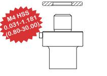
Precision ground punch shim returns the NEXT punch assembly to the original length after 0.118(3.00) has been removed during routine regrinding.
